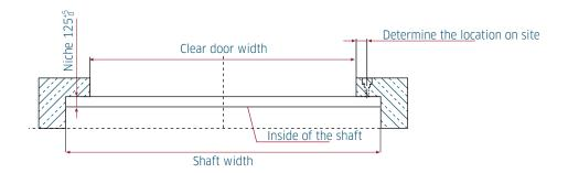
Door threshold / edge protection passable with axle load over the entire opening width, by others!
