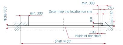
Door threshold / edge protection passable with axle load over the entire opening width, by others!
