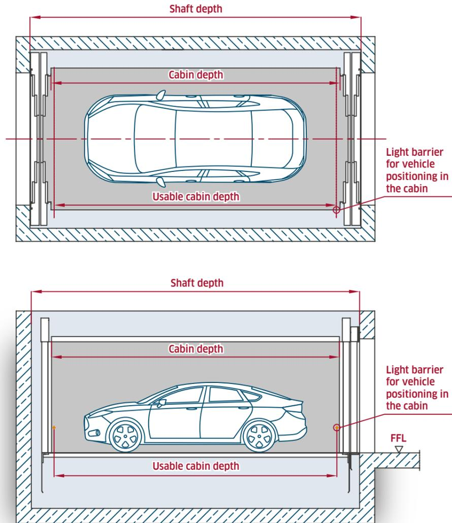
In the case of car lifts **with a front- and rear-opening design**, the dimensions are as follows.\*
